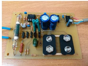
Output voltages can reach  $\pm 120$  V. Minimal detected current is 1 pA. The input and output circuits are isolated (floating), which allows working with  $\mu$ SEM structures of any configuration (detector or cathode at ground potential). A diagram of an example  $\mu$ SEM setup and close-up photo are shown below.
