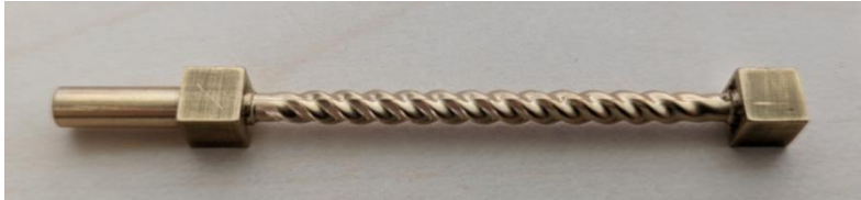
First trials milling a mandril at 94 GHz
