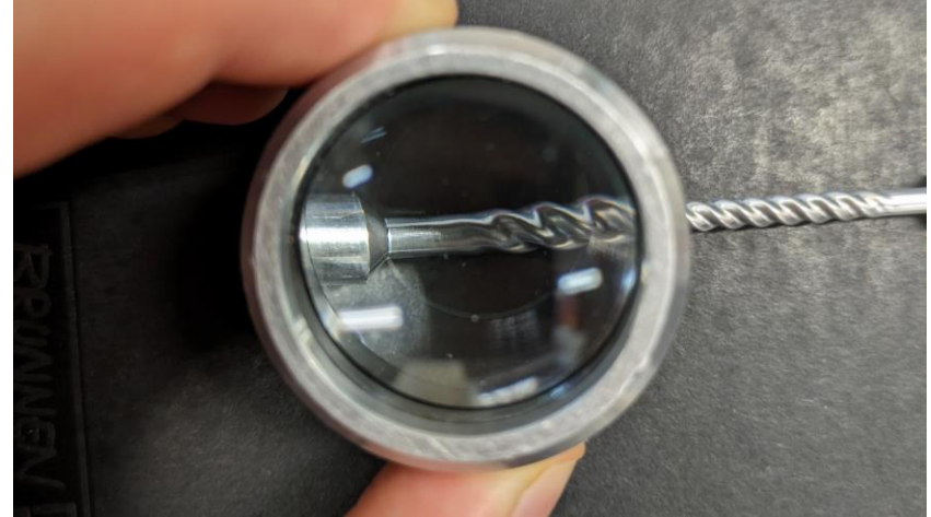
Mandril for the first electroplating trials at 94 GHz
