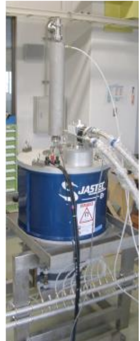
The appearance of FU CW IIB gyrotron
