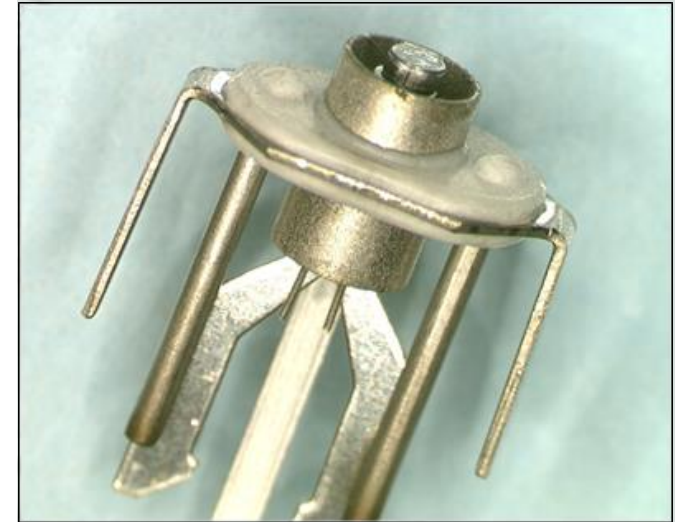
Philips 0,65 Watt I cathode unit as used in the tests
