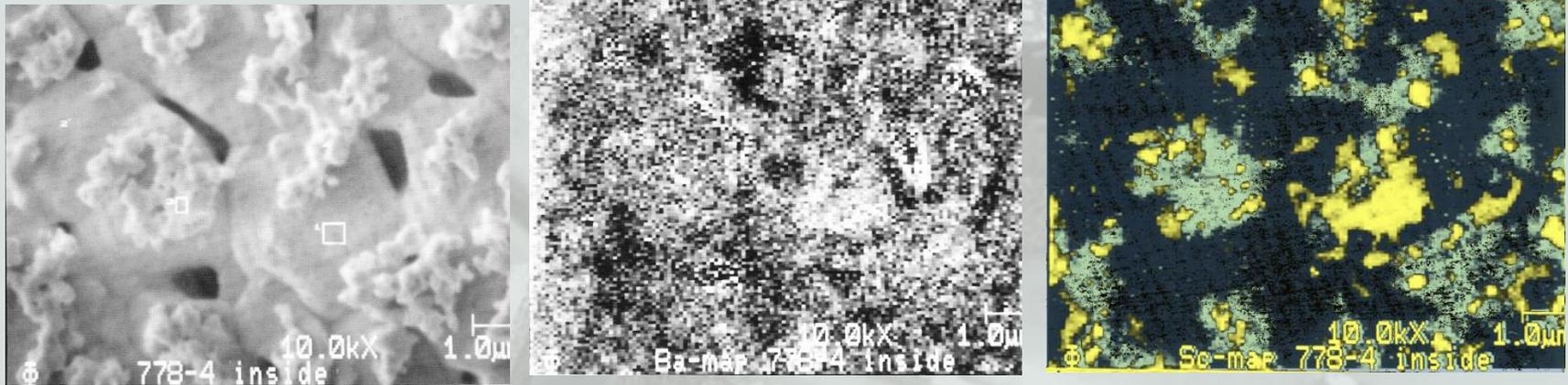
a) SEM micrograph (above) of **LAD top layer Scandate cathode** in the central beam emitting region **after ion bombardment**; the cathode was re-activated for 30 min at  $1060^{\circ}\text{C}_{\text{Mo-Br}}$  and then kept at  $965^{\circ}\text{C}_{\text{Mo-Br}}$  during SAM [4].
