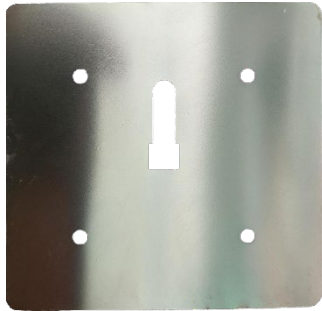
Shadow-mask for the coating process (laser- cutted stainless steel sheet)
